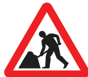
7001 Road works or temporary obstruction on carriageway ahead
